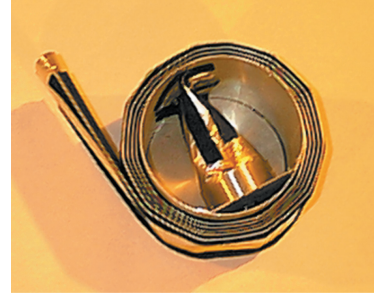
Fig. 2 A 5-m STR boom rolled up on a 0.165-m-diam mandrel.
